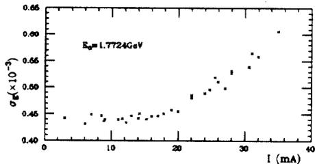
Fig.1 Energy Spread Measurements
