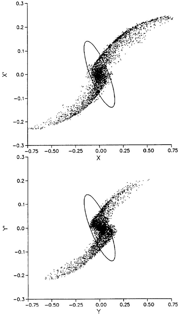
Figure 1. Experimental particle distributions (in cm and mrad) from the einzel lens LEBT. The design specification beam emittance ellipse is shown.
