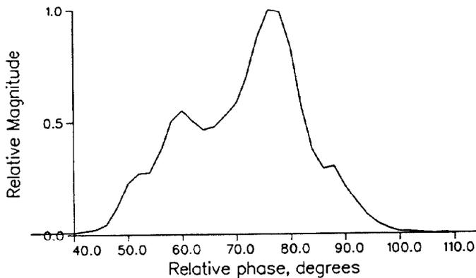
Figure 4. Measured longitudinal phase signal from the bunch shape monitor.
