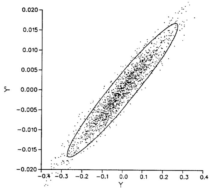
Figure 2. Transverse ( $y$ - $y'$ ) particle plot in cm and mrad of simulated output beams at the slit position.
