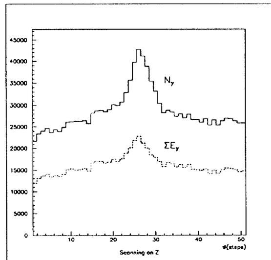
Figure 2: Angular scan around Z axis for scintillator ( $N_\gamma$ ) and calorimeter ( $\Sigma E_\gamma$ )
