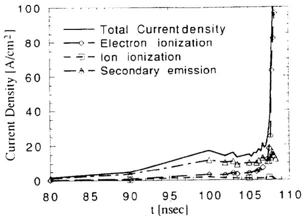
Figure 1: Total electron current density at the anode and its components versus time. The system parameters are  $p = 2$  torr,  $V_0 = 20$  kV,  $d = 1$  cm and an initial plasma density of  $5 \times 10^7 / \text{cm}^3$ .
