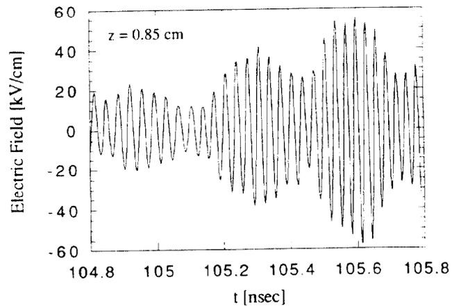
Figure 3: The electric field at  $z = 0.85$  cm versus time. Note the growing plasma oscillation. Same system parameters as in Fig. 1.
