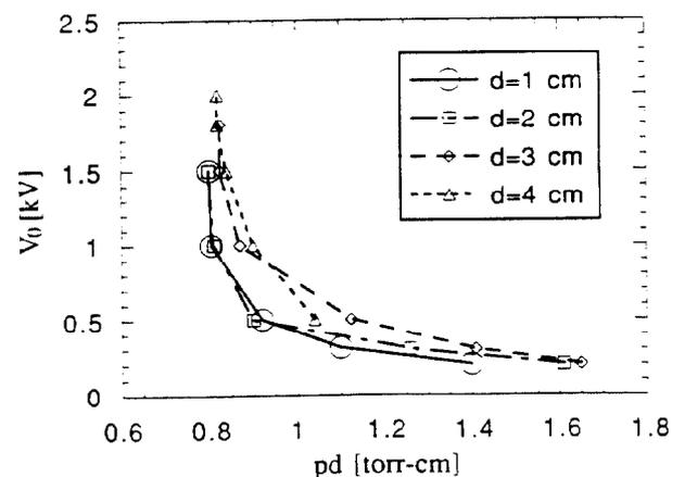
Figure 5: Breakdown Voltage as a function of gas pressure times gap length for gap lengths from 1 to 4 cm.
