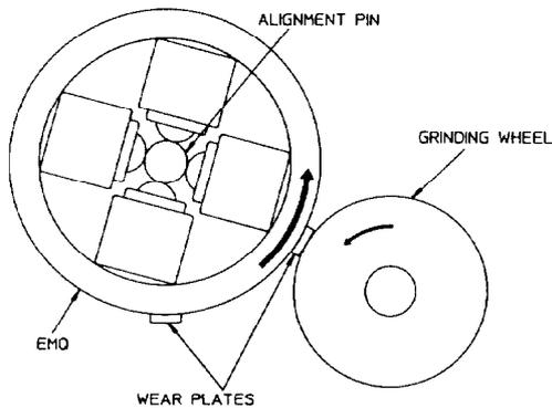
Fig. 5. Grinding EMQ Wear Plates.
