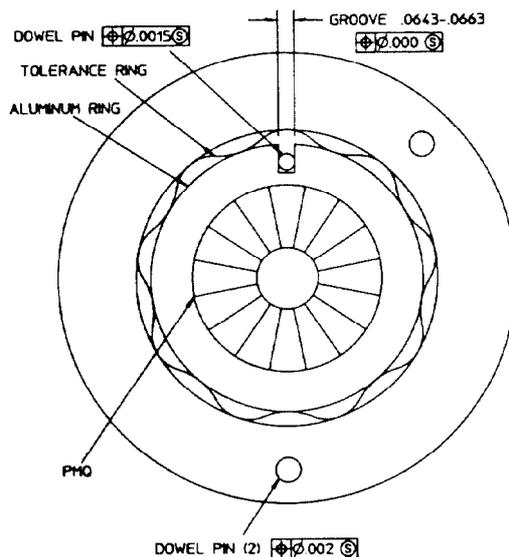
Fig. 3. PMQ and Holder Assembly.
