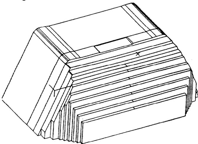
Figure 2: Isometric drawing of the final endpack design.
