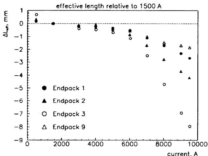
Figure 1: Effective length (relative to 1500 A) vs current for endpacks #1, original straight cut; #2, stepped approximation to straight cut; #3, Borda profile; and #9, Rogowski profile.
