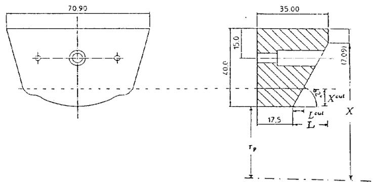
Figure 2: Profiles for pole-end chamfers
