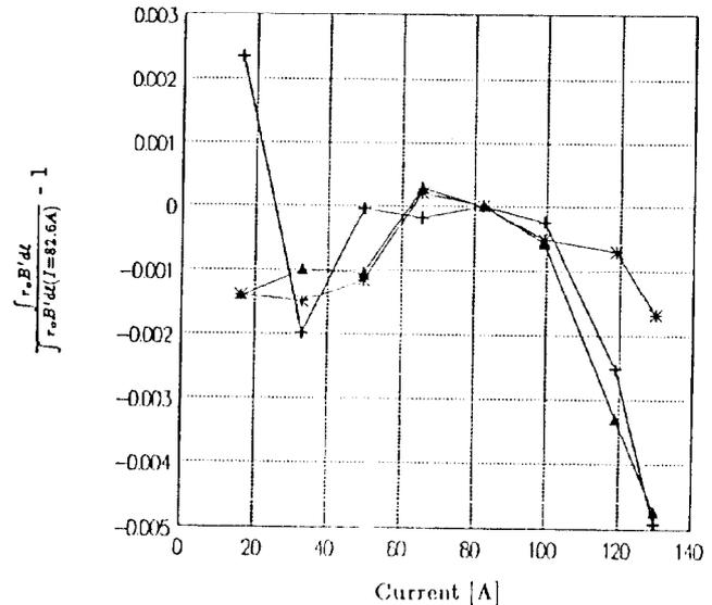
Figure 4: Difference in normalized  $\int r_o B' dl$  versus current: Normalized at  $I=82.6$  A. \*; as assembled,  $\Delta$ ; chamfered and shimmed Q1, and +; chamfered and shimmed Q2.
