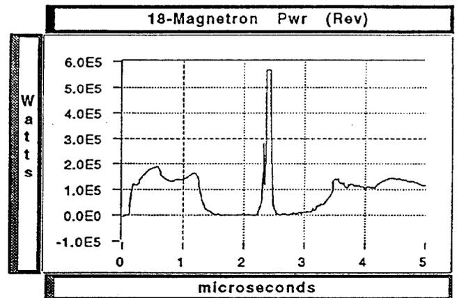
Fig. 3. Magnetron's reflected power signal (power flowing from the input cavity toward the magnetron). The spike at 2.3  $\mu$ s is the result of the electron reflection in the upstream direction from the output cavity.
