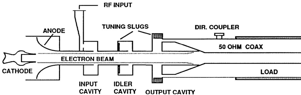
Fig. 1. Schematic diagram of the RKA.
