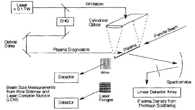
Figure 1: Outline of Plasma Lens Experimental Setup
