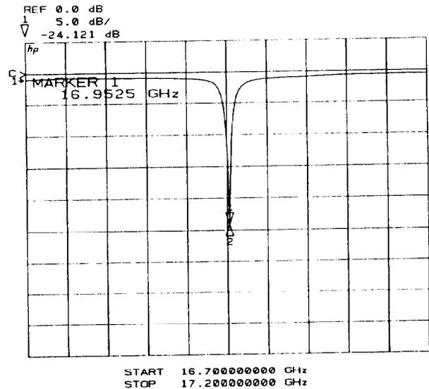
Fig.4: Reflected Power as a function of frequency of a tuned gun structure
