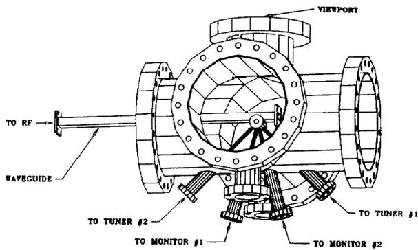
Fig.2: RF Gun Vacuum chamber. The gun structure is located at the center of the chamber.
