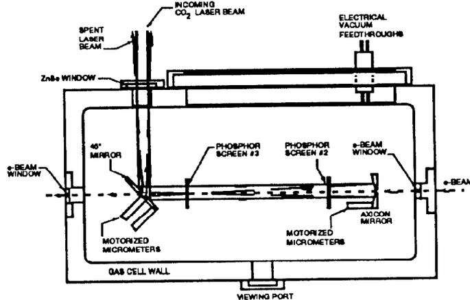
Figure 4. Schematic plan view of gas cell.
