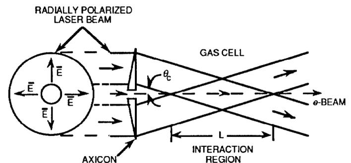
Figure 1. Basic arrangement for inverse Čerenkov acceleration.
