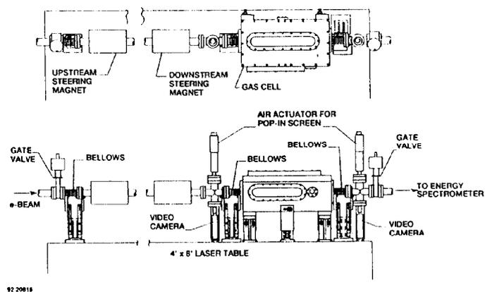
Figure 3. Schematic of ATF ICA beamline system.
