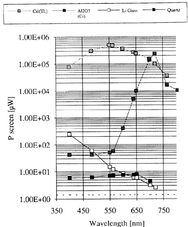
Fig. 3: Spectral emission curves of four screen materials
