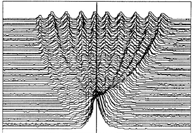
Figure 1: Mountain range plot of high intensity beam during the bunch rotation phase of coalescing. Note that the earlier bunches are debunching while the later ones preserve their shape.
