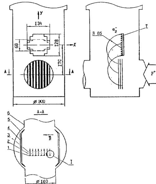
Fig.1. Layout of the beam monitor.
