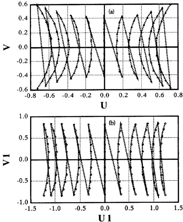
Fig. 9 Calculated response of the SOR-RING's BPM
