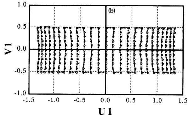
Fig. 7 Measured response of the SOR-RING's BPM
