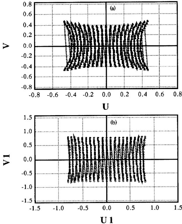
Fig. 8 Calculated response of the cylindrical BPM
