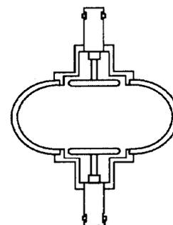
Fig. 2 Cross-sectional view of a pair of ion-clearing electrodes
