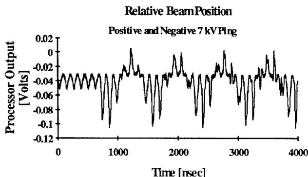
Figure 1: Coherent Beam Motion after a 7-kV Ping
