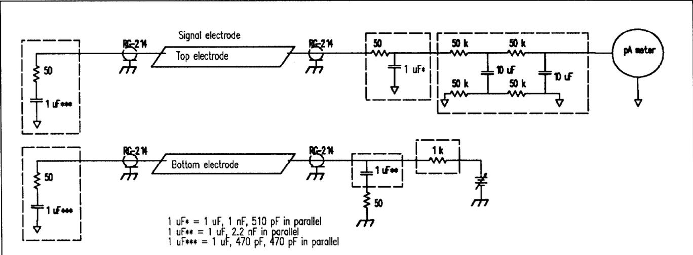
Figure 3: Pinger Electrode Connection for use as an Ion Chamber
