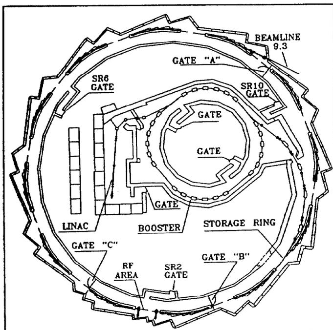
Figure 1 - ALS Floor Plan
