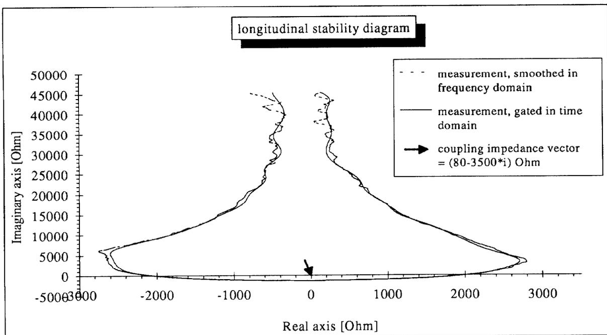
Figure 5. In this "stability diagram" the beam response of figure 1 and figure 4 is shown in the complex plane rather than in an amplitude and phase diagram. The effect of time gating becomes important at low particle numbers and low excitation strength.
