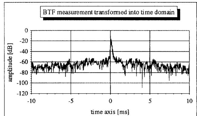
Figure 2. The inverse Fourier transform of the BTF represents the beam response to an impulse excitation.
