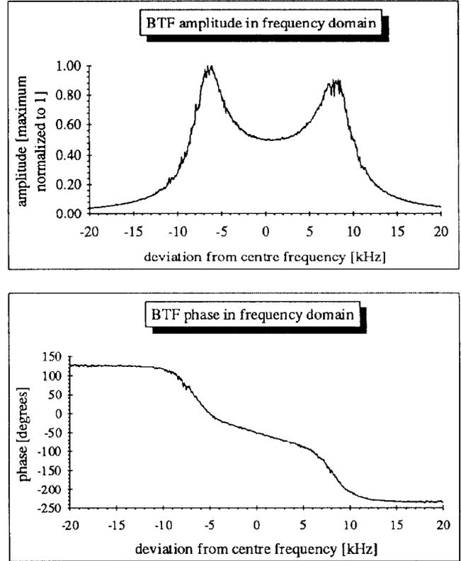
Figure 1.  $S(\omega)$  of a longitudinal BTF measurement with a coasting beam of  $7.6 \cdot 10^9$  protons at 200 MeV/c in LEAR, revolution frequency = 0.796 MHz, centre frequency = 42.17 MHz,  $(\Delta p / p)_{FWHM} = 1.6 \cdot 10^{-4}$
