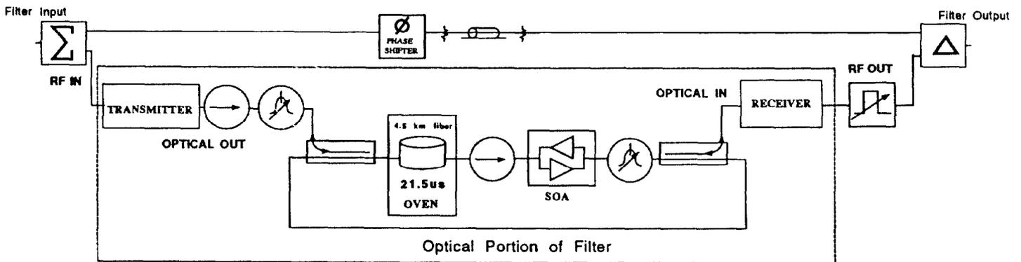
Figure 6. Block diagram of optical storage ring correlator notch filter
