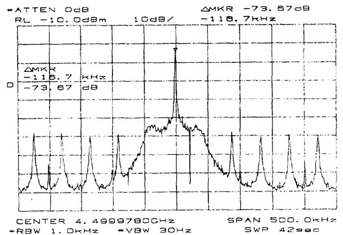
Figure 9. Dynamic range performance of actual filter. Filter is narrow band swept by network analyzer and plotted on wide band with spectrum analyzer. Peaks are noise floor of optical portion of correlator filter.
