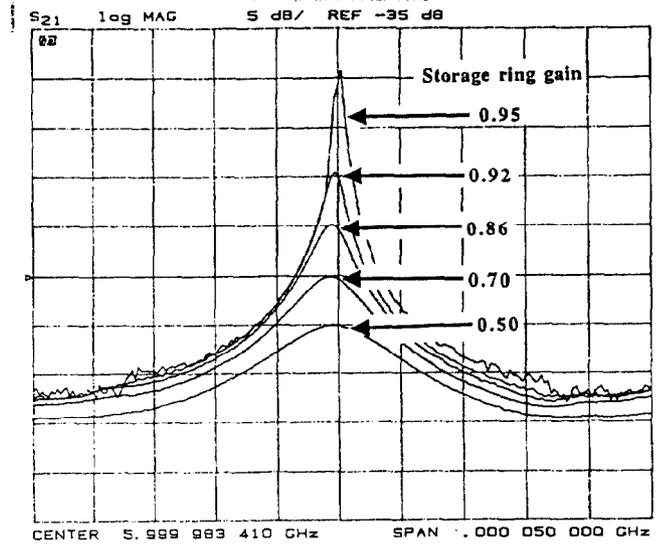
Figure 7. Variation of optical storage ring Q as a function of loop gain.
