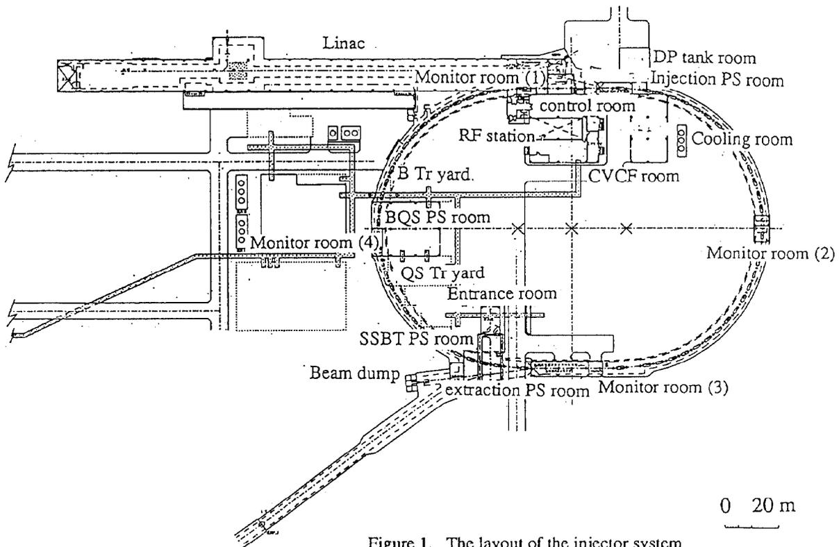
Figure 1. The layout of the injector system
