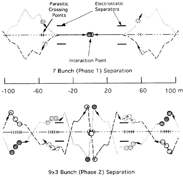
Figure 2. Pretzel separation plan near the IR. The present 7 bunch layout is shown in the top view. The 9x3 bunch train with a  $\pm 2.5$  mrad horizontal crossing angle is shown in the bottom view. The scales' aspect ratio is highly distorted.
