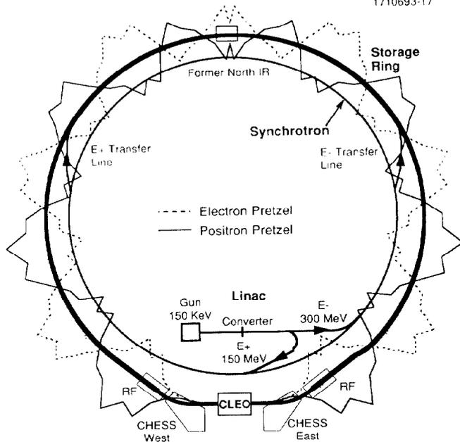
Figure 1. Schematic layout of CESR and injector complex. Pretzel orbits for 7 bunch operation are superimposed on the CESR ring.
