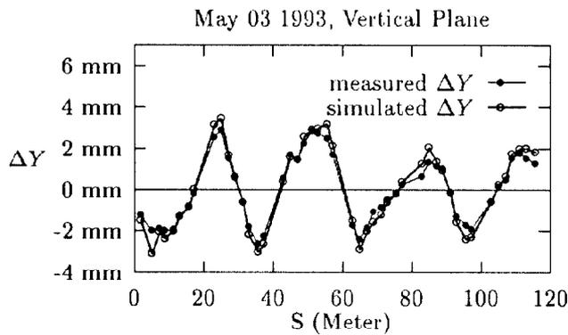
Figure 5: Comparison of the measured  $\Delta Y$  and simulated COD change by the correctors with specified strengths.
