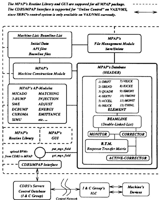
Figure 1: The structure of SRRC/Beam Dynamics Group's MPAP.
