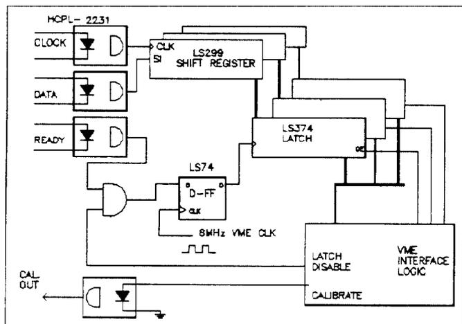
Figure 2. VME block diagram
