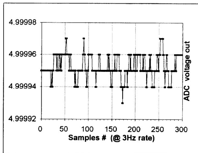
Figure 3. Noise measurement. Input to ADC is 5V.
