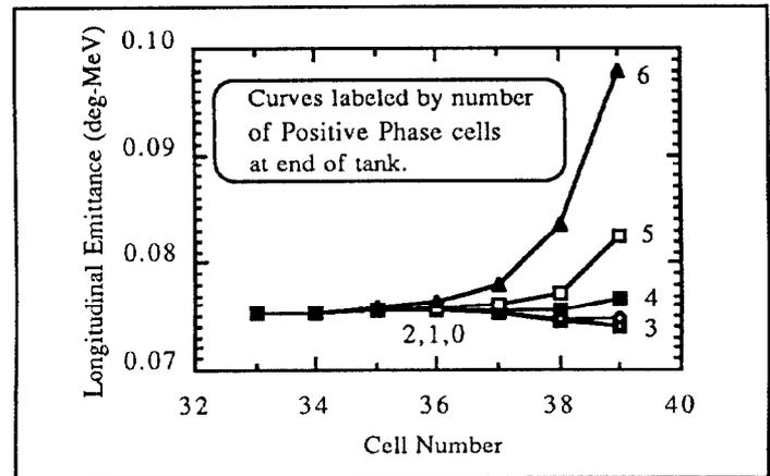
Figure 4. Effect of Positive Phasing on Beam Performance
