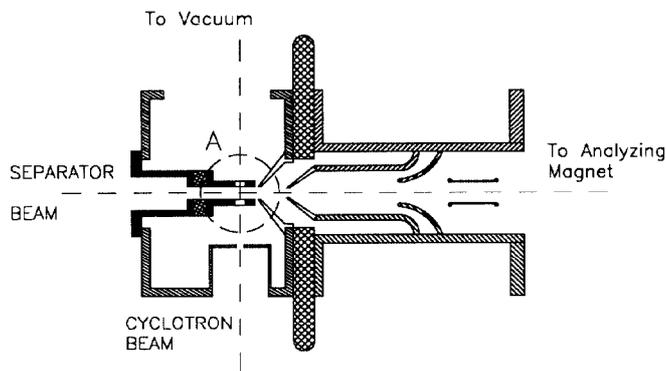
**Fig. 2** Schematic drawing of the modified Jvaskylä ion guide used as the special Target Ion Source.
