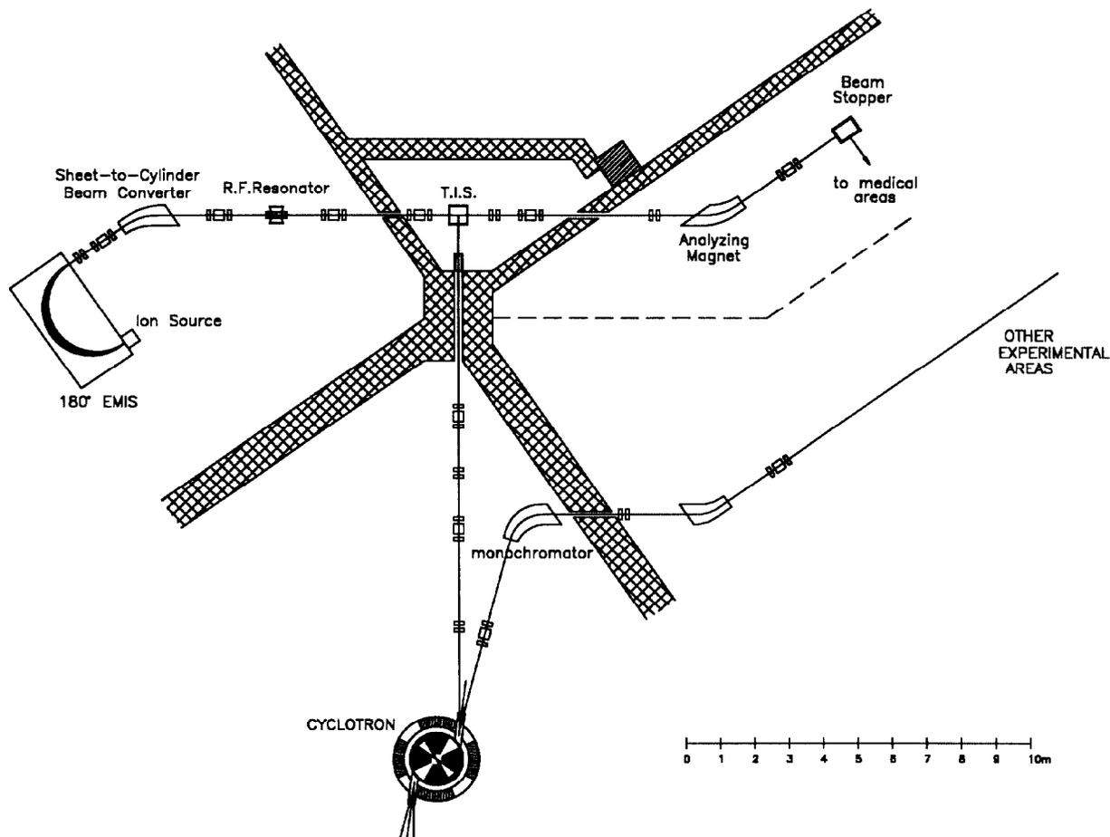
**Fig.1** General layout of the new EMIS-CYCLOTRON scheme for production of PET nuclides
