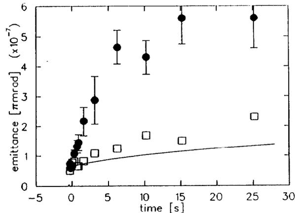
Figure 5: Experimental horizontal ( $\bullet$ ) and vertical ( $\square$ ) blow-up of 21 MeV protons, measured at  $7 \mu\text{A}$ .
