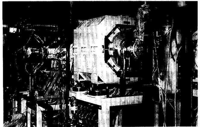
Figure 1: *The ferrite loaded quadrupole resonator.*
