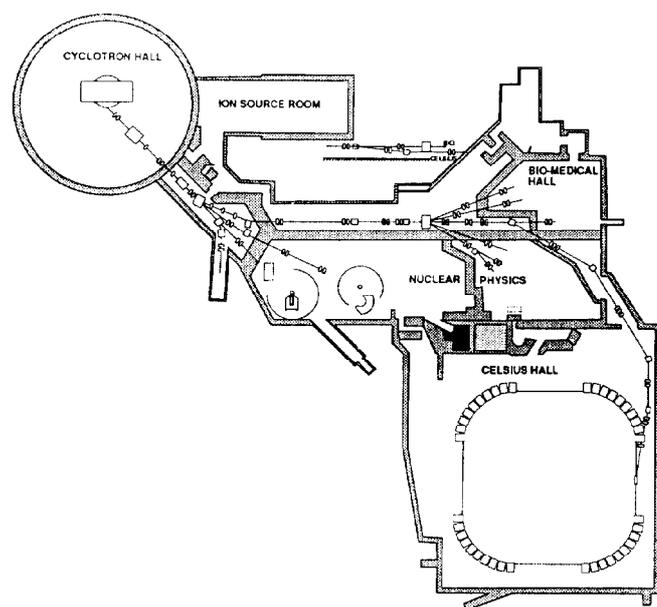
Fig. 1. The Gustaf Werner cyclotron complex. The CELSIUS ring has a circumference of 82 m.
