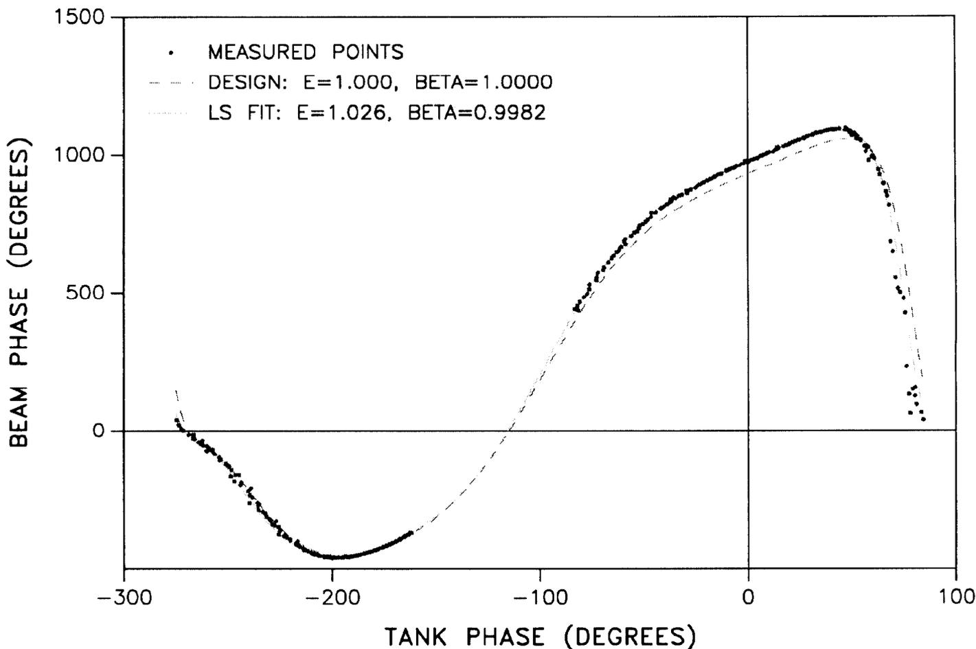
Figure 2. Phase-scan curves for tank 6 of the Fermilab drift-tube linac. Beam phase is measured 16.96 meters past the end of tank 6. Tank electric field ( $E$ ) and beta (at input) are referenced to design values.
