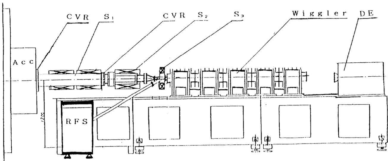
$S_1, S_2$ : Beam transport solenoid coil, RFS: Radio-Frequency Source,
