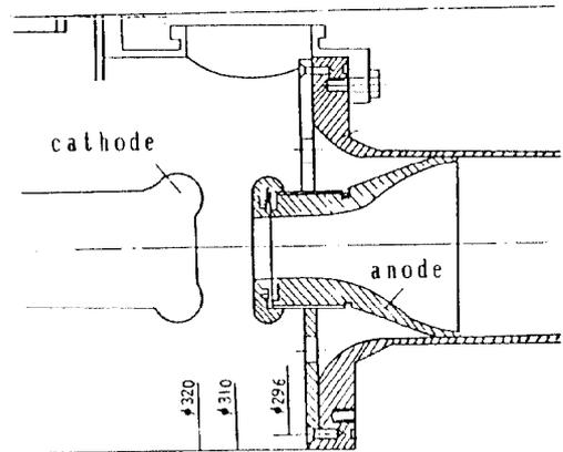
Fig. 2 The cross section of injector
