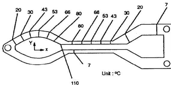
Figure 3. Temperature Rise due to Beam Missteering (Case 2)
