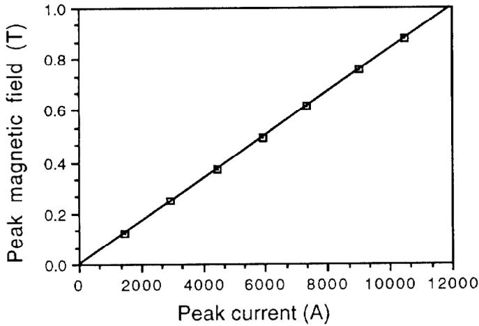
Figure 8. Peak magnetic field vs. peak current.
