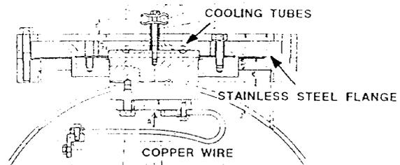
Figure 7. The septum magnets cooling system.
