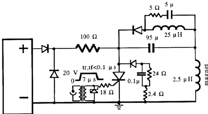
Figure 3. Power pulse circuit
