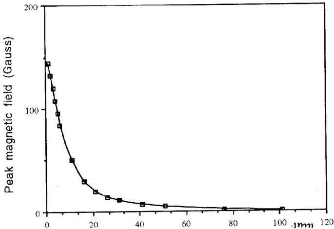
Figure 10. Peak magnetic field vs. distance from the septum.
