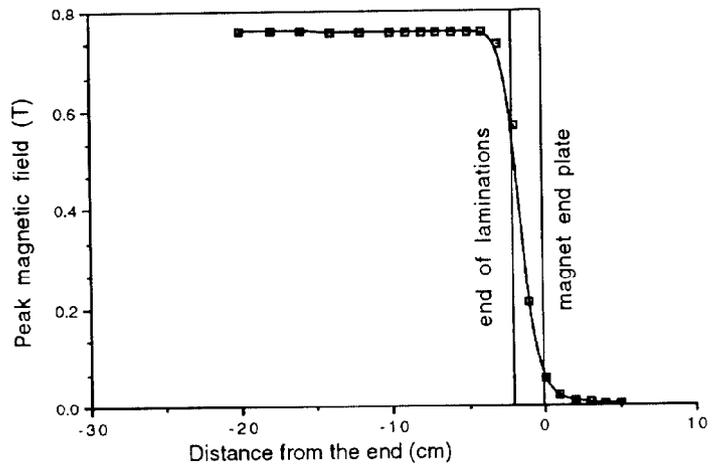
Figure 11. Peak magnetic field along the longitudinal axis.
