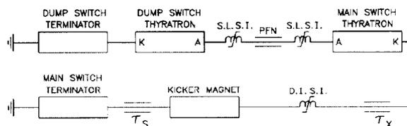
Figure 1: Block diagram of pulse generator and magnet
