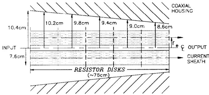
Figure 2: CERN PS Division Resistive Terminator
