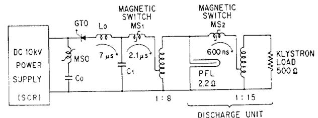
Figure 1. Simplified diagram of the all-solid-state klystron modulator.
