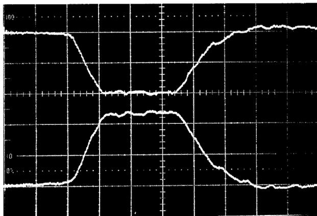
Figure 4. Output pulse waveforms at the dummy load.
