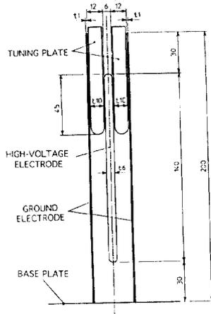
Figure 2. Cross section of the PFL.
