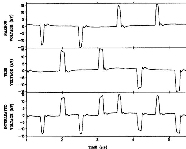
Figure 3: Measured wide, narrow and inter-leaved pulse patterns.
