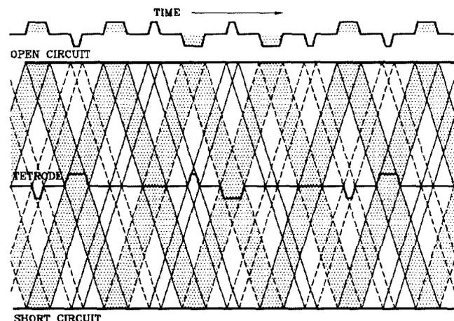
Figure 2: Lattice diagram of inter-leaved chopper pulses.
