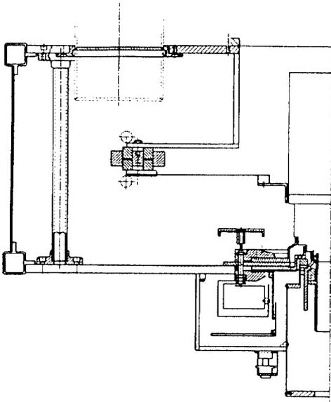
Figure 2. Scale drawing of the final cavity with the Thomson TH-535 tube installed.
