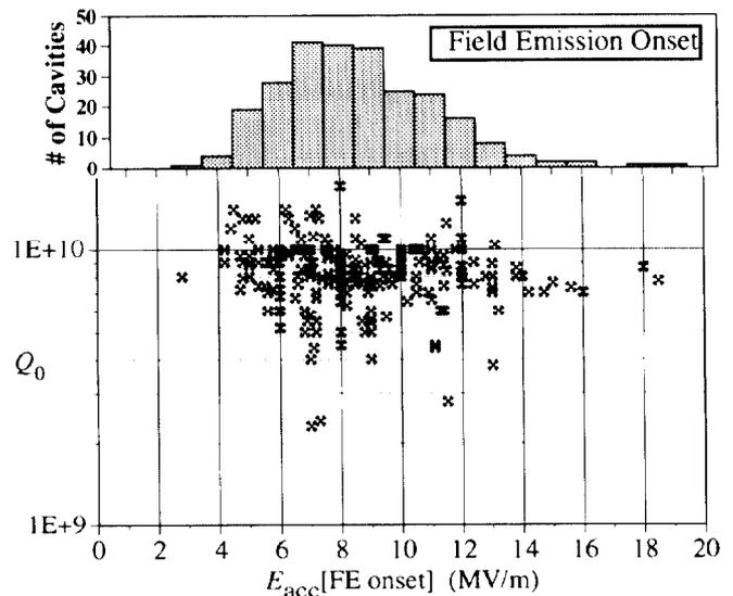
Figure 3.  $Q$  and gradient at onset of field emission loading.
