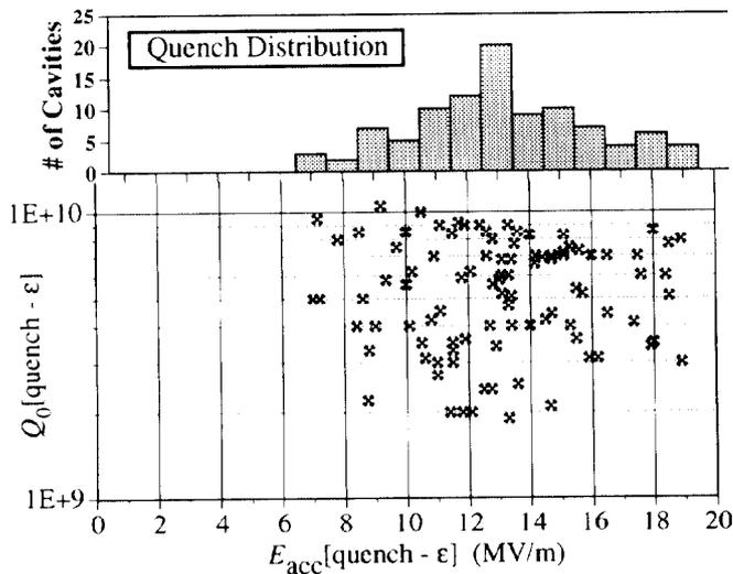
Figure 5. Cavity  $Q$  and gradient just below quench.
