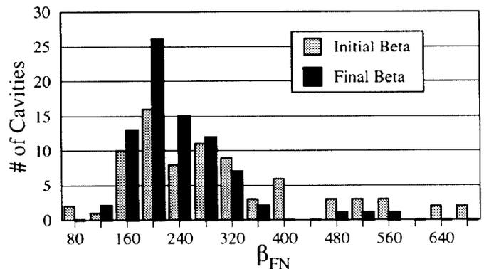
Figure 4. Field enhancement factors for FE limited cavities.
