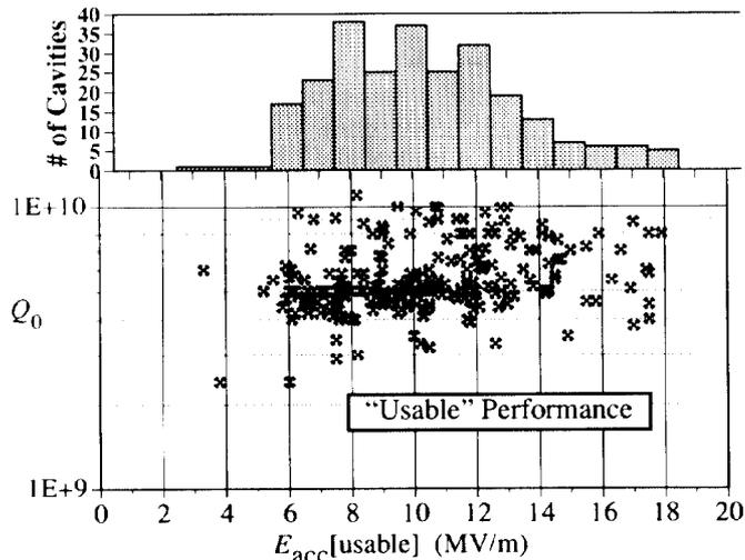
Figure 2. Cavity  $Q$  factor at maximum "usable" gradient.
