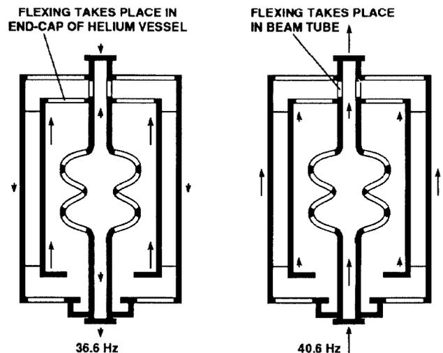
Figure 2. Longitudinal mechanical modes associated with the helium vessel. Only longitudinal motion is shown.
