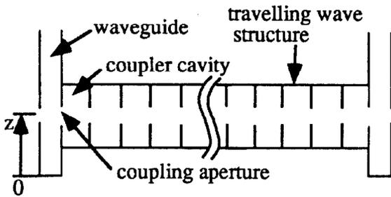
Figure 3: Electric coupling
