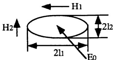
Figure 1: Coupling aperture
