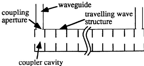
Figure 2: Magnetic coupling
