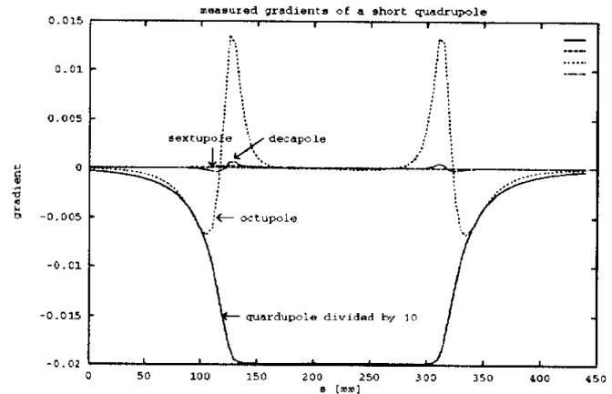
Figure 10: Example of measured gradients of a short quadrupole [4]
