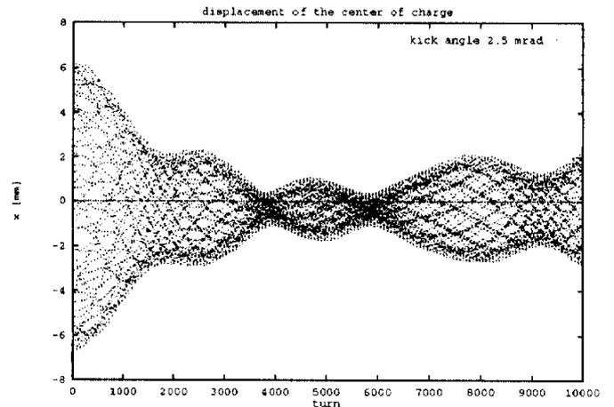
Figure 6: Displacement of the center of charge versus turn for 2.5 mrad kick
