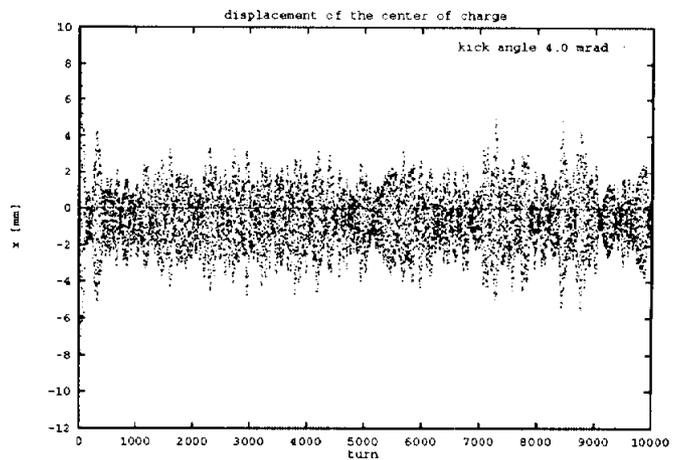
Figure 7: Displacement of the center of charge versus turn for 4 mrad kick
