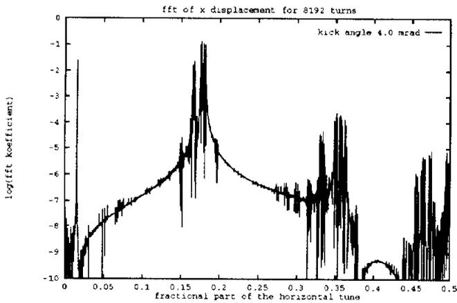
Figure 9: fft of the displacement with 4 mrad kick
