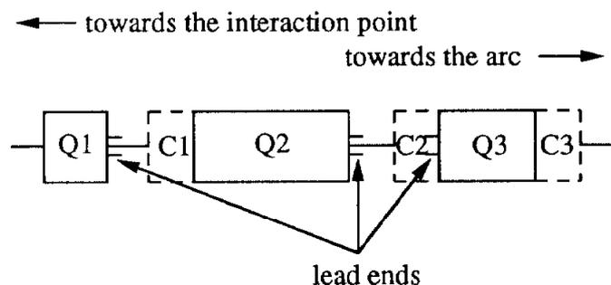
Figure 1 Schematic layout of the RHIC triplet, showing the quadrupoles, the orientation of the quadrupole lead ends, and the local correctors C1, C2, and C3 .
