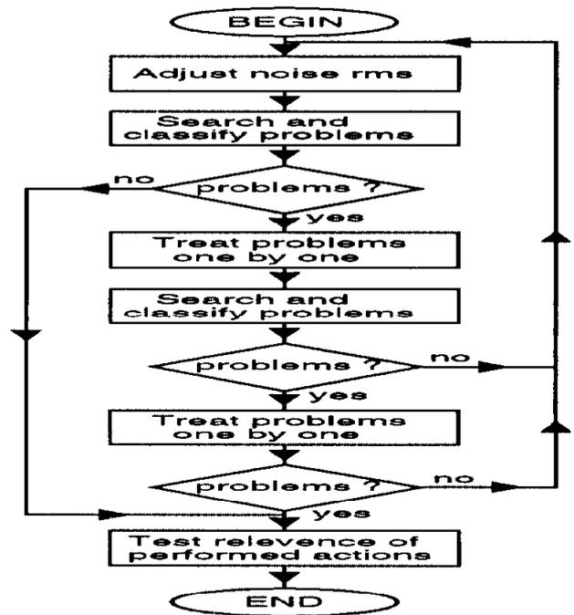
Figure 1: Automatic orbit treatment algorithm
