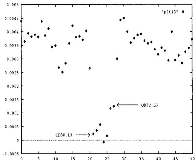
Figure 2: Misalignment missed by the fitting method. This misalignment makes a series of  $\pi$ -bumps if the phase advance per cell is  $90^\circ$ , which is the case for the named quadrupoles.
