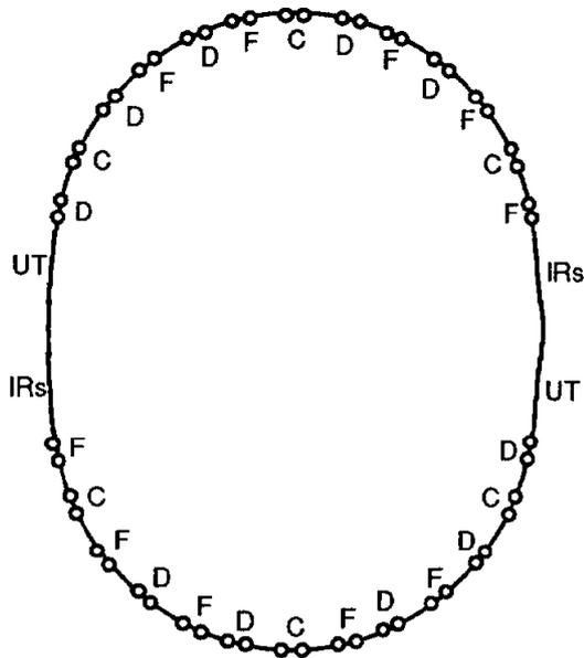
Figure 1. Sketch showing the approximate layout of the 15 m free spaces in the arcs of the Collider; the polarities shown are of the nearest quad in the upper ring.
