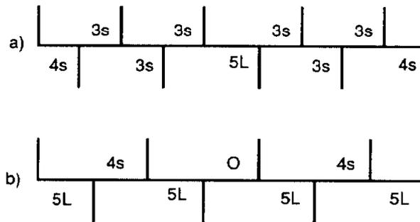
Figure 2. (a) 1990 design of bending region between two IRs within a cluster. (b) New design of this region, generating a high dispersion point in the middle half cell. The number of 13 m (s) and 15 m (L) dipole magnets in each half cell are indicated.
