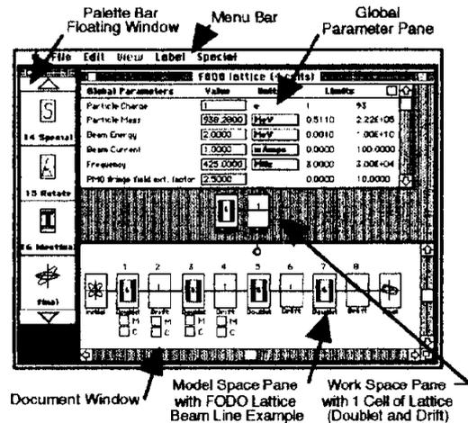
Figure 1. TRACE 3-D SPARC Application Screen.
