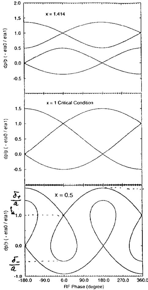
Figure 1: The stationary bucket near transition. The vertical axis is momentum offset normalized to  $a = -\frac{\eta_0}{\eta_1}$ .
