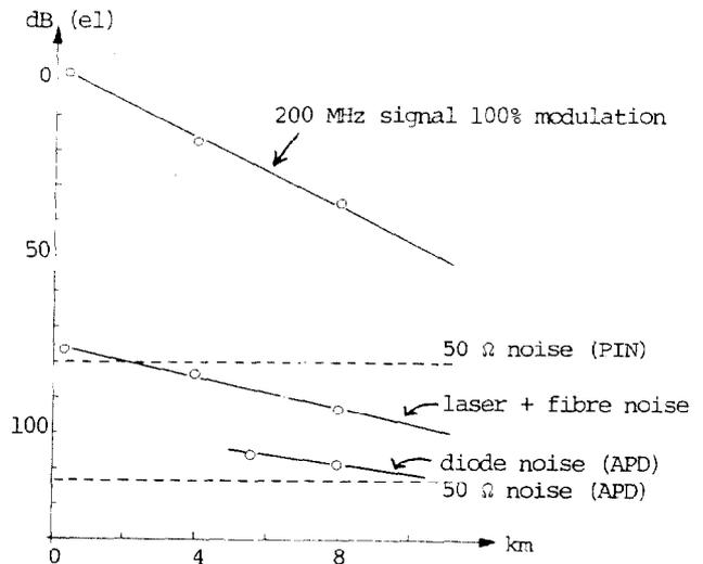
Fig. 3 Relative signal and noise levels (10 kHz BW)
