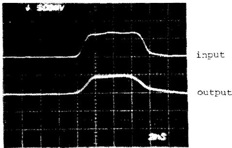
Fig. 2 Pulse transmission over 8 km (2ns/div)
