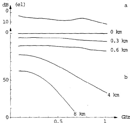
Fig. 1 Laser-receiver (a) and fibre (b) transfer functions
