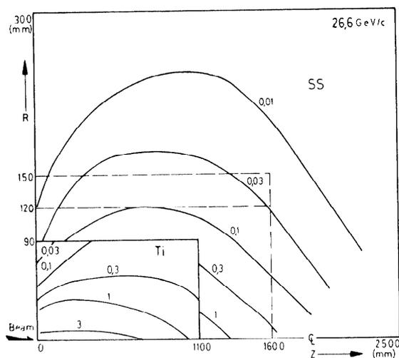
Fig. 2 Energy Deposition Density [MeV cm<sup>-3</sup> per proton]
