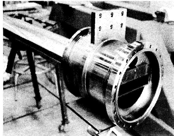
Fig. 4 Front Part of the Vacuum Chamber With the Copper Collimator in Place
