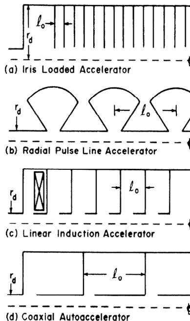
Fig. 1—Schematic Accelerator Diagrams
