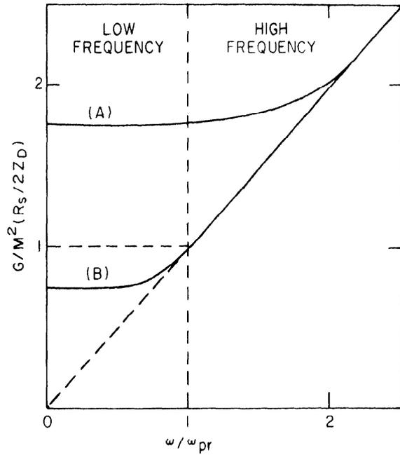
Fig. 2—Variation of the Gain function for the longitudinal bunching mode of the klystron instability.
