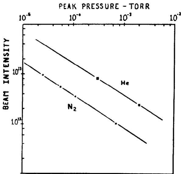
Fig. 3. The threshold for beam blowup is plotted as a function of peak pressure and beam intensity for localized pressure bumps of  $N_2$  and He; above the lines the beam is unstable. A higher peak pressure of He is tolerated by the beam than for  $N_2$ .
