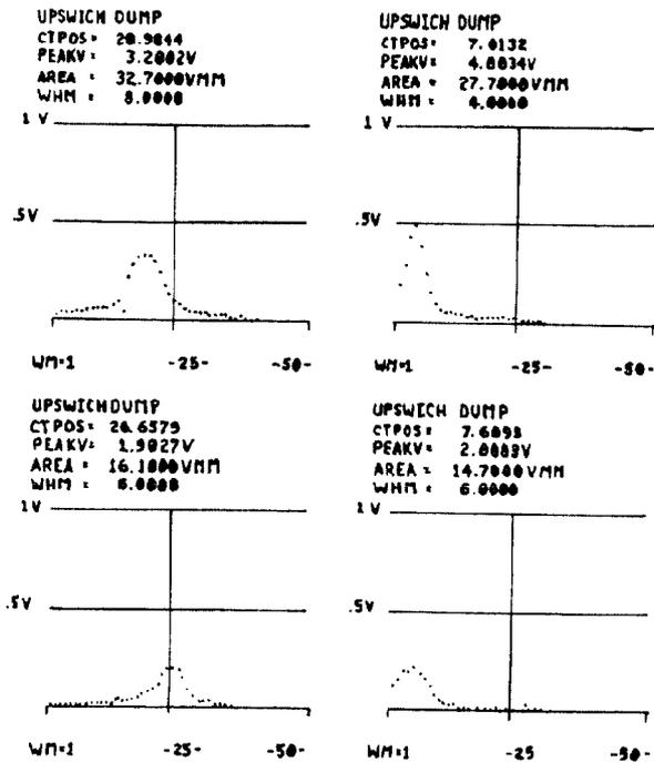
Fig. 5. The extracted beam profile, as measured at the main ring dump, is measured both horizontally (left) and vertically (right). The upper plots are taken with no jet and the lower plots are taken on a cycle when the jet was pulsed. The most striking difference between the two measurements is the change in the horizontal position of the extracted beam indicating a possible tune shift.
