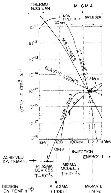
Fig. 1. Reaction parameter  $\langle\sigma v\rangle$  for various losses and gains as a function of beam energy for head-on collisions.
