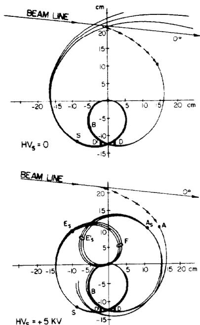
Fig. 8. Computer generated orbits fit to observed interceptions of beam by probe. Upper and lower plots are for non-linear kicker off and on, respectively.
