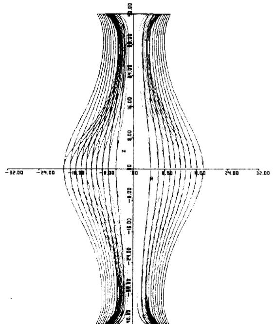
Fig. 4. Magnetic flux lines compared with the more sharply curved migma energy envelopes for the same magnetic field. (See text).
