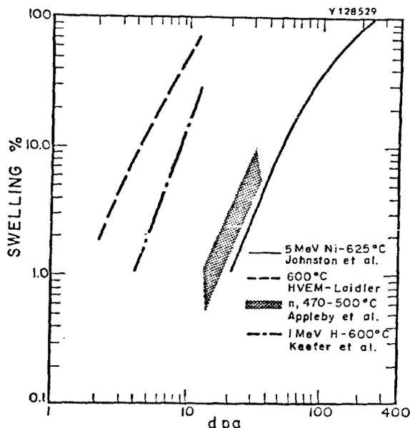
Fig. 3. Comparison of neutron-induced swelling in 316 stainless steel to that determined by  $H^+$ ,  $Ni^+$ , and HVEM simulation studies.<sup>10</sup>
