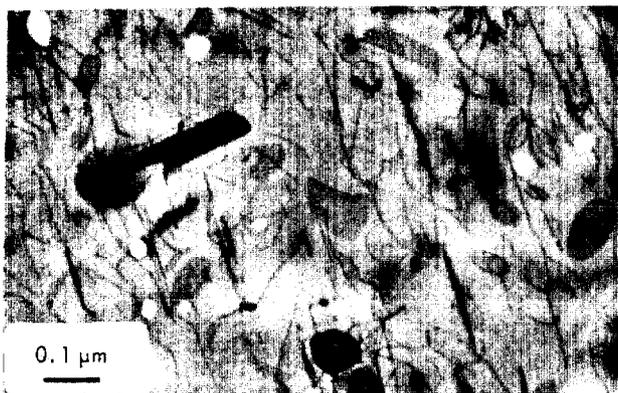
Fig. 1. Transmission electron micrograph showing voids and interstitial dislocation loops in type 316 stainless steel irradiated to  $2 \times 10^{22}$  n/m<sup>2</sup> in EBR-II.
