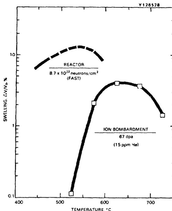
Fig. 2. Temperature dependence of swelling in annealed-type 316 stainless steel bombarded with 5-MeV nickel to a damage level of 67 dpa. The steel contained 15 ppm of cyclotron-injected helium. The temperature dependence of EBR-II core swelling is shown by the dashed curve. The displacement rates were  $\sim 10^{-6}$  dpa/sec in EBR-II and  $2 \times 10^{-2}$  for the ion bombardment. (Johnson et al.<sup>9</sup>)
